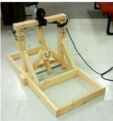
After construction, it was necessary to test the design. Using energy based mathematics it was approximated that the catapult would launch a water balloon approximately 65 to 70 feet with an increased angle. Testing proved this result to be accurate within about 3 feet of the desired target.
